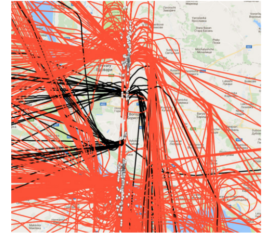
Figure 47: Black lines highlight performed visual approaches that can save 28 kg per landing on the E190.
